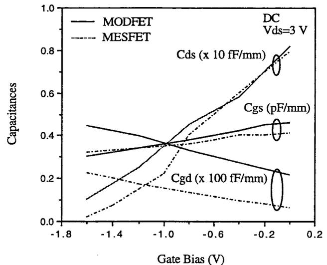
Fig. 13. Variations of gate-source capacitance  $C_{gs}$ , feedback capacitance  $C_{gd}$ , and drain-source capacitance  $C_{ds}$  with gate bias for MODFET and MESFET using quasi-static approach.
