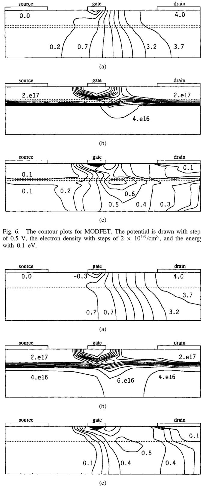
Fig. 6. The contour plots for MODFET. The potential is drawn with steps of 0.5 V, the electron density with steps of  $2 \times 10^{16} / \text{cm}^3$ , and the energy with 0.1 eV.
