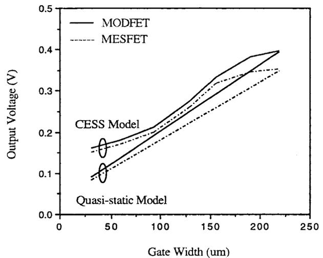
Fig. 10. The comparison of output voltage variations with device width obtained from the CESS model and the quasi-static model for MODFET and MESFET.
