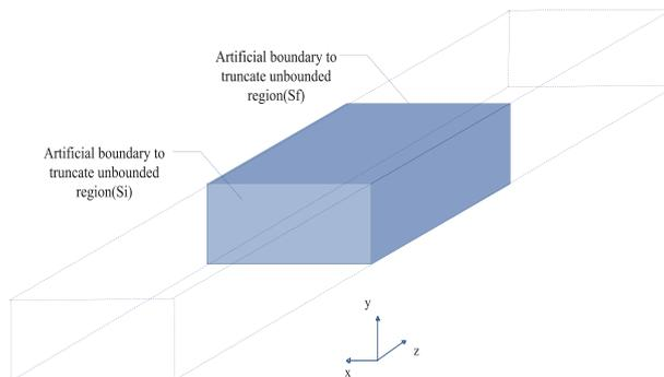
Figure 4. The rectangular waveguide and its artificial boundary condition (absorbing boundary condition).
