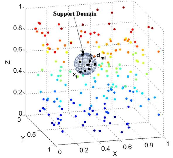
Fig. 1. The support domain for a point  $\mathbf{x}_i$  in the mesh-free method.
