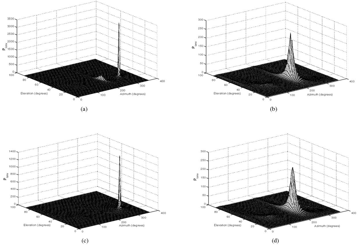
Fig. 1.  $P_{lcmv}(\theta, \phi)$  function at sequential iterations of DMSAE method: (a)-(d) corresponding to iterations 1-4
