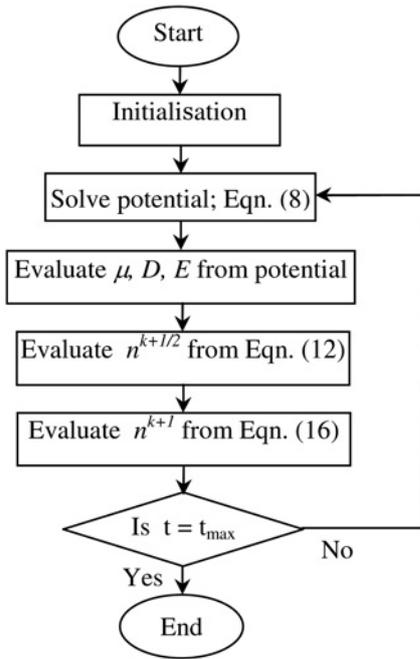
**Fig. 1** Flowchart of the sequence of LOD-FDTD scheme for the DDM
