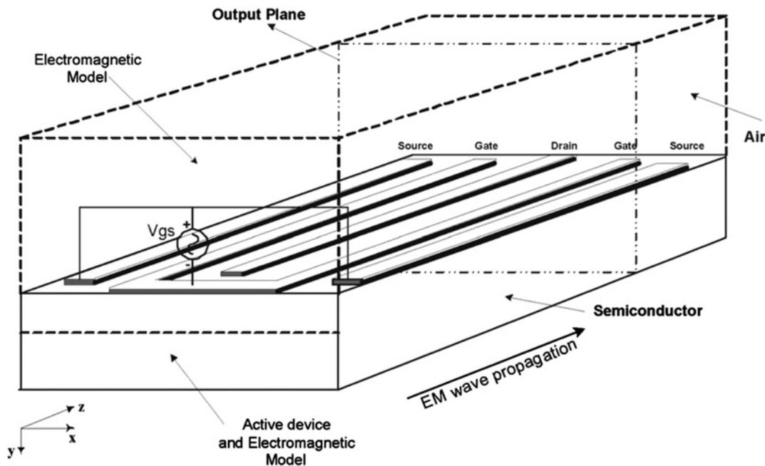
Fig. 13 Simulated two-finger MESFET structure
