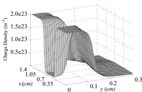
Fig. 3 Carrier density distribution from LOD-FDTD DC simulation
