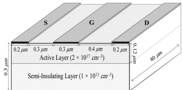
**Fig. 2** Simulated MESFET structure
