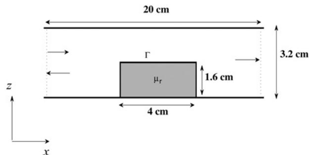
**Fig. 7** Magnetic material rod inserted in a parallel-plate waveguide
