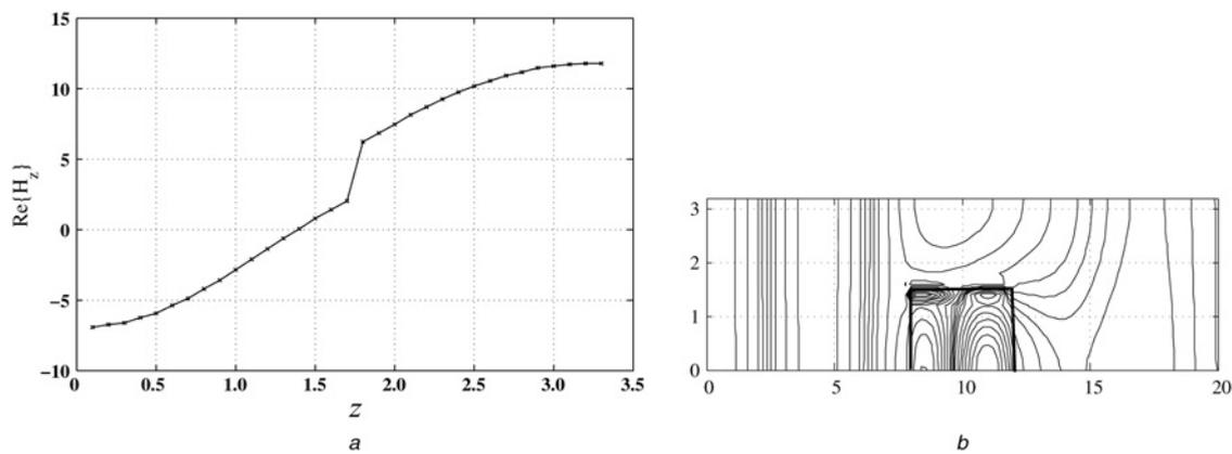
**Fig. 8** Field in the parallel plate waveguide with a magnetic material rod
