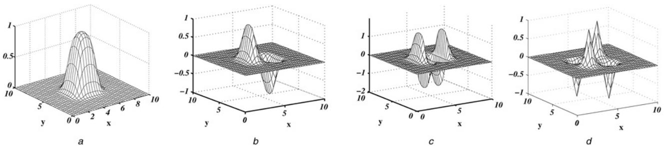
**Fig. 1** Proposed shape function and its derivatives on a (5 × 5) uniform node distribution for one of the middle nodes
