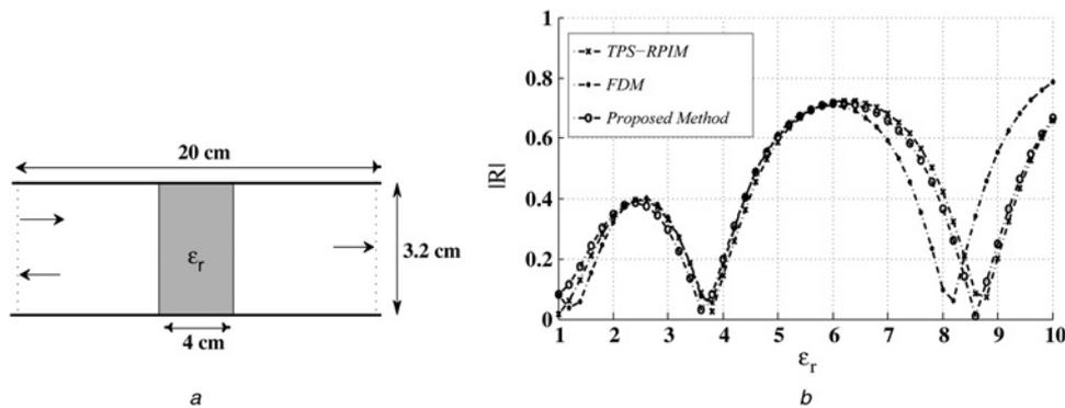
**Fig. 6** Parallel-plate waveguide with dielectric material rod
