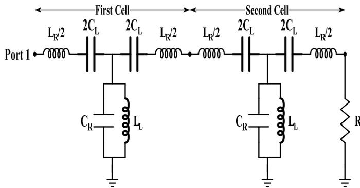
Figure 3. Suggested antenna: equivalent circuit model contributed of the symmetrical two unit cells.
