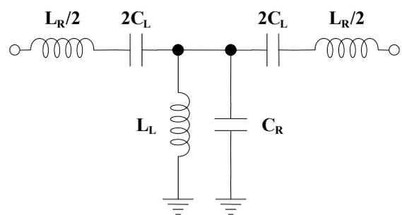
Figure 1. Proposed Antenna: equivalent circuit model for composite right/left-handed transmission line of the one unit cell.
