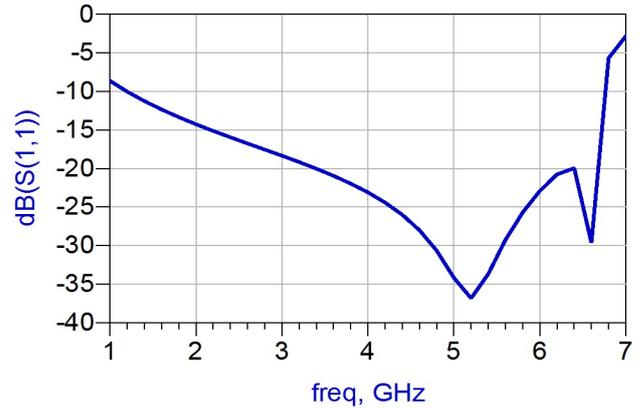
Figure 4. Simulated  $S_{11}$  parameter.
