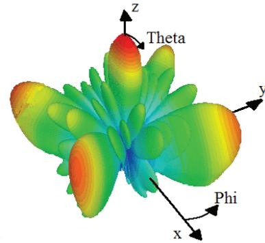
Fig. 11. 3-D radiation pattern of the planar array designed using proposed configuration in [4].
