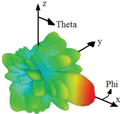
Fig. 10. 3-D radiation pattern of the planar array designed using the proposed configuration in this paper.
