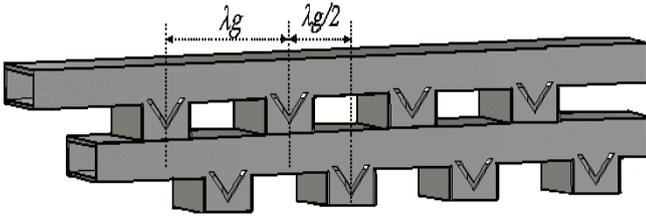
Fig. 2. Planar array with the effective slot spacing equal to  $\lambda_g/2$  and close to  $\lambda/2$ .
