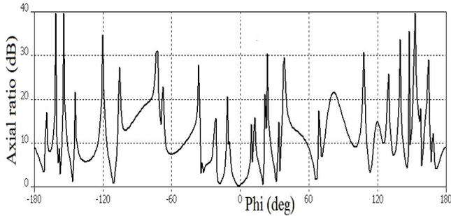
Fig. 5. Axial ratio of the linear array versus  $\phi$  in the  $xy$  plane.
