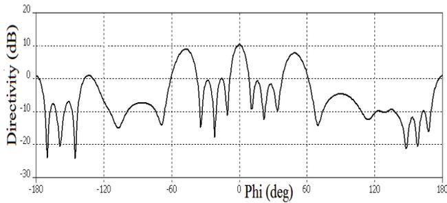
Fig. 6. Directivity of the linear array versus  $\phi$  in the  $xy$  plane.
