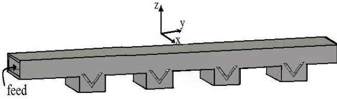
Fig. 4. Linear array with four radiating v-slots.
