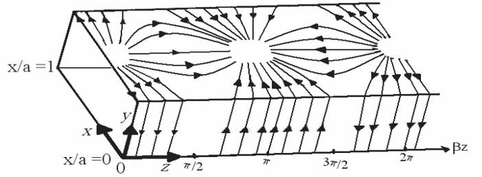
Fig. 3. The current distribution on the interior walls of the waveguide.
