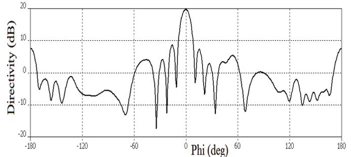
Fig. 9. Directivity of the planar array versus  $\phi$  in the  $xy$  plane.
