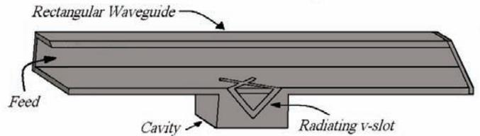
Fig. 1. Proposed waveguide slot antenna configuration.
