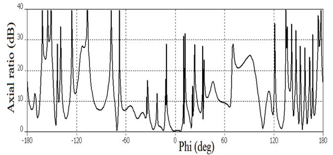
Fig. 8. Axial ratio of the planar array versus  $\phi$  in the  $xy$  plane.
