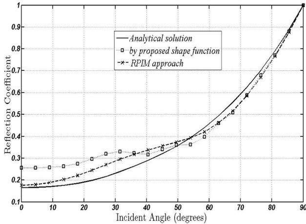
Fig. 4. Reflected coefficient of the metal-backed dielectric slab.
