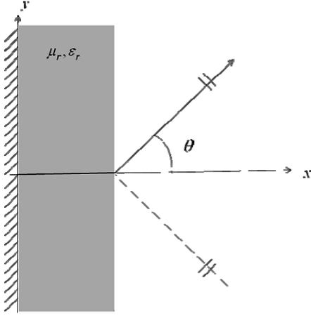
Fig. 3. Plane wave reflected by a metal-backed dielectric slab.
