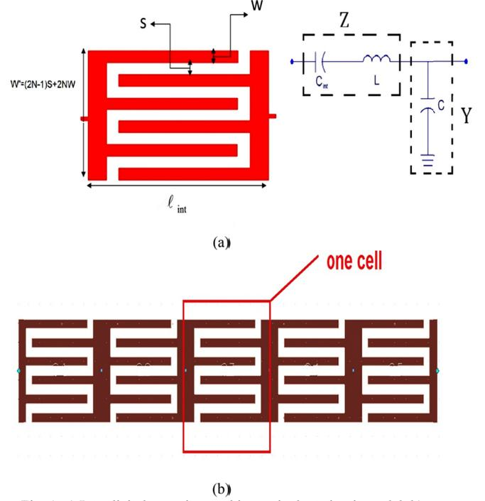
Fig. 1. a) Interdigital capacitor and its equivalent circuit model. b) Interdigital TL
