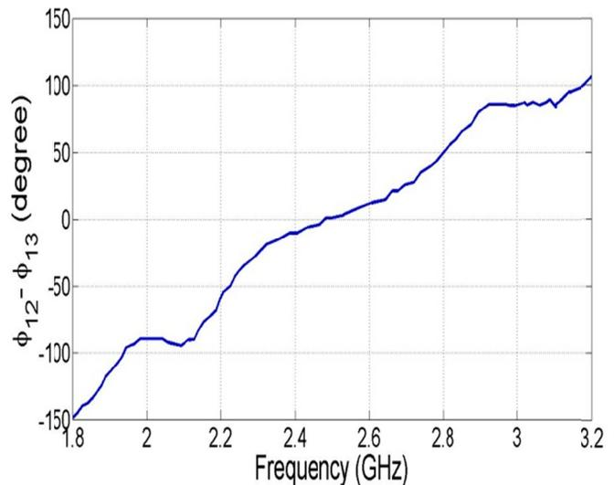
Fig. 4: Simulated phase difference between the through and coupled ports for the proposed coupler of Fig. 2.
