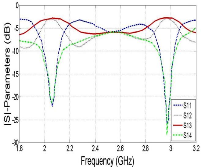
Fig. 3: Simulation results of the proposed DB branch-line coupler (on FR4 substrate with 1.6 mm thickness and  $\epsilon_r = 4.8$ )
