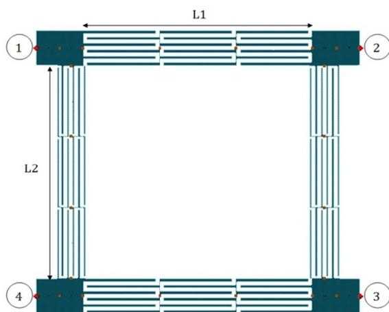
Fig. 2: Layout of the proposed dual-band branch-line coupler
