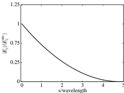
**Figure 3.** Electric field in vicinity of paramagnetic scatterer.
