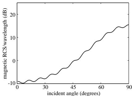
**Figure 8.** Backscattered RCS for magnetic field in vicinity of paramagnetic scatterer.
