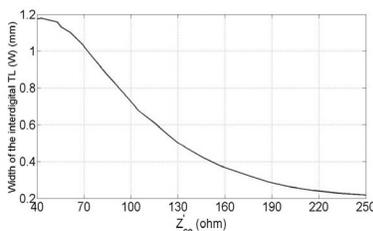
**Figure 3.** Width of the interdigital TL ( $W$ ) in the proposed coupler versus  $Z'_{ce}$  on FR4 substrate,  $\epsilon_r = 4.7$ , thickness of 1.6 mm.
