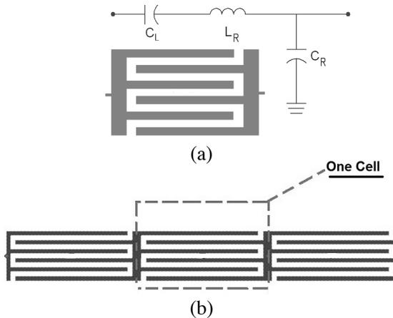
**Figure 1.** (a) Interdigital capacitor and its equivalent circuit model. (b) Interdigital transmission line (TL).
