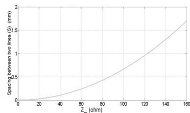
**Figure 4.** Spacing between two coupled interdigital TLs ( $S$ ) in the proposed coupler versus  $Z_m$  on FR4 substrate,  $\epsilon_r = 4.7$ , thickness of 1.6 mm.
