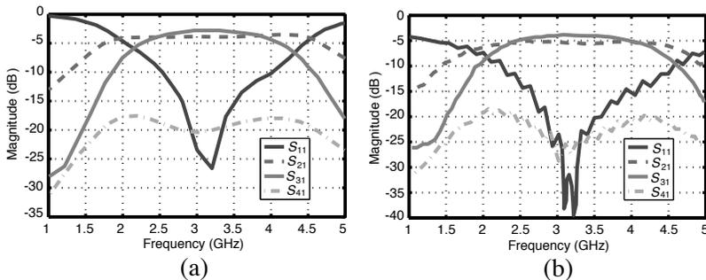
**Figure 5.**  $S$ -parameters of the proposed coupler shown in Figure 2. (a) Full-wave simulation results. (b) Measurement results.
