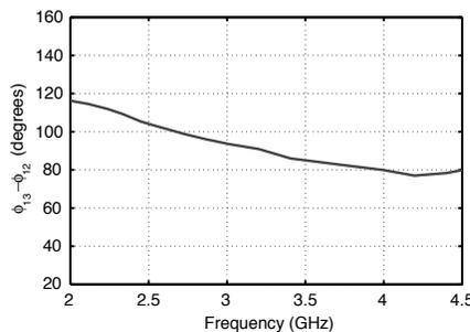
**Figure 6.** Measured phase difference between the through port and the coupled port for the proposed coupler of Figure 2.
