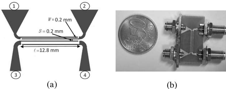
**Figure 2.** Structure of the proposed microstrip coupled-line backward coupler on FR4 substrate,  $\epsilon_r = 4.7$ , thickness of 1.6 mm. (a) Structure layout. (b) Fabricated coupler.
