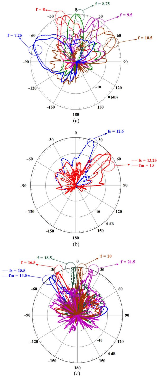
Fig. 9. Measured and simulated radiation patterns of the proposed antenna. Solid line: measurement results (fm). Dash line: simulation results (fs). (a) First CRLH band. (b) New RH band. (c) Second CRLH band.
