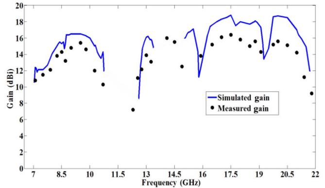
Fig. 6. Measured and simulated gains of the antenna.
