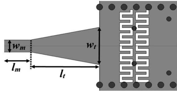
Fig. 2. Tapered microstrip feed line for impedance matching.
