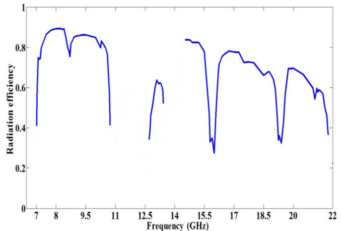
Fig. 7. Simulated radiation efficiency of the proposed LWA.
