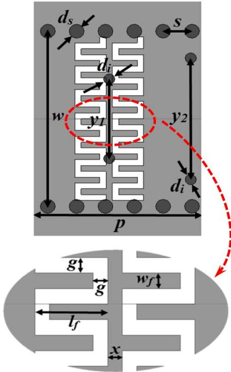
Fig. 1. Unit cell of the proposed SIW CRLH LWA.
