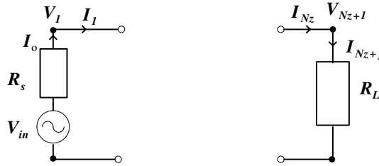
Figure 4. Discretization of the terminal voltages and currents.
