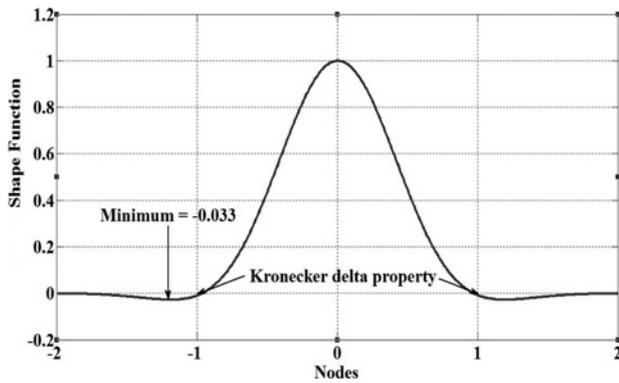
Fig. 6 Proposed shape function for wave equation at  $f = 3$  GHz and  $\Delta x = 0.01$
