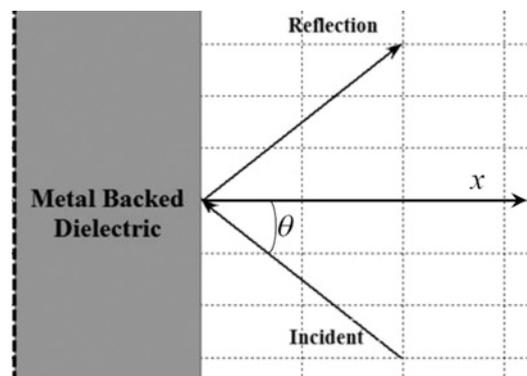
**Fig. 5** Problem domain of the incident wave on a metal backed dielectric
