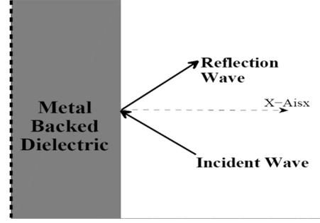
Fig. 1. Problem domain of the incident wave on a metal backed dielectric.
