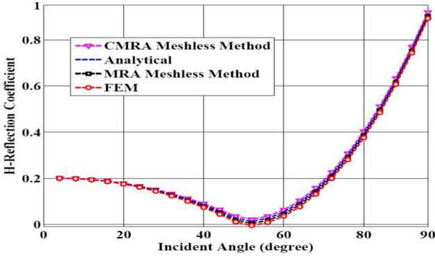
Fig. 3. Reflection coefficient of magnetic polarization at  $f = 3$  GHz using different methods.
