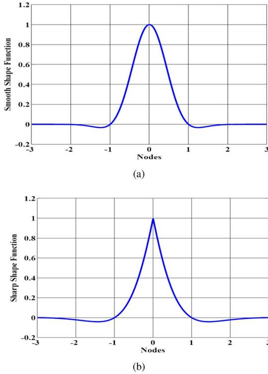
Fig. 2. Proposed (a) smooth and (b) sharp shape functions for wave equation at  $f = 3$  GHz.
