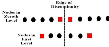
Fig. 4. CMRA discretization used for analyzing the incident wave problem with  $J_{\max} = 1$  as the maximum level of resolution.
