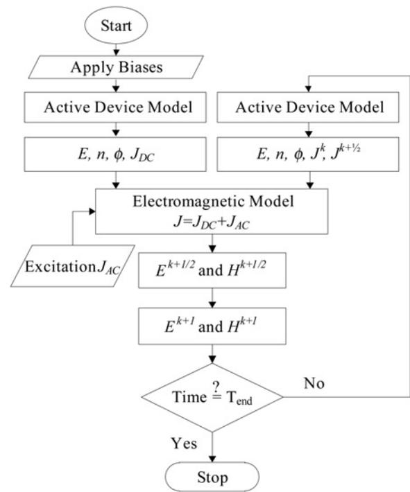
Fig. 1 Flowchart of the sequence of full-wave simulation of a semiconductor device
