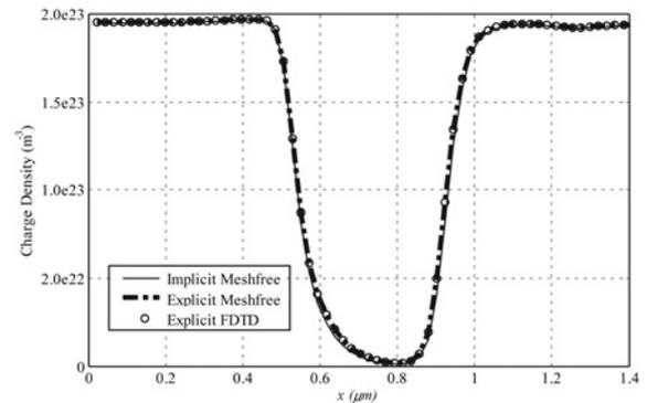
Fig. 4 Charge density across the 'x'-direction at 'y = 0.09  $\mu\text{m}$ ' for different methods
