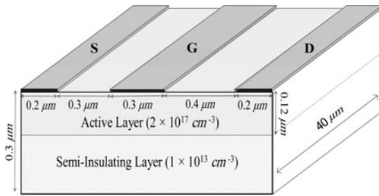
Fig. 2 Simulated MESFET structure
