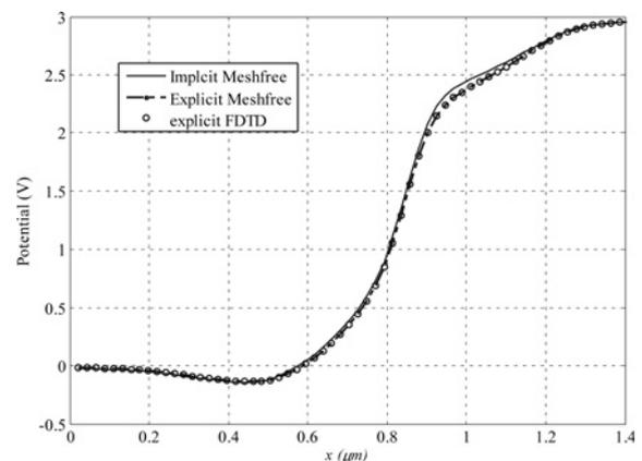
Fig. 5 Potential distribution across the 'x'-direction at 'y = 0.09  $\mu\text{m}$ ' for different methods
