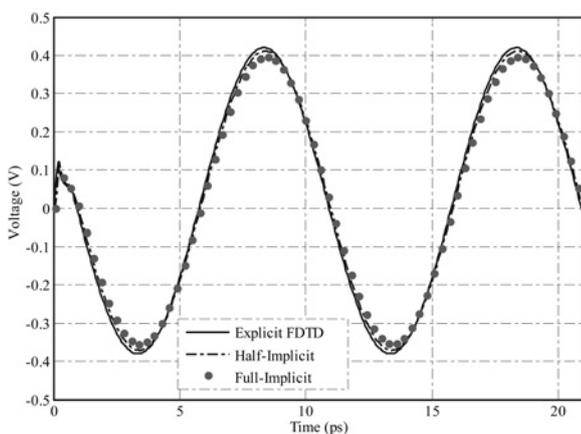
**Fig. 6** Output drain voltage from explicit FDTD ( $\Delta t = 0.01$  fs), half-implicit ( $\Delta t = 1$  fs) and full-implicit ( $\Delta t = 10$  fs) methods
