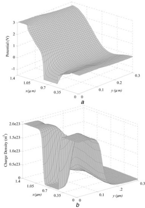
Fig. 3 DC simulation results by the proposed algorithm
