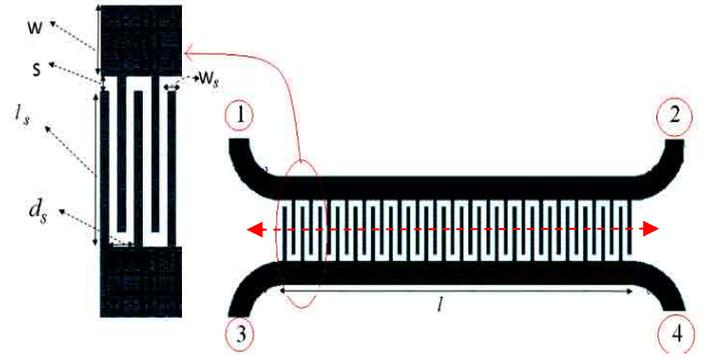
Fig. 1. Proposed forward coupled-line coupler structure with periodic stubs.
