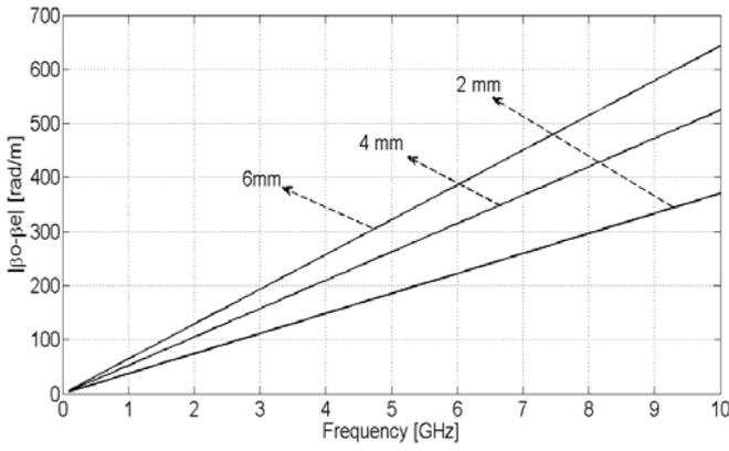
Fig. 4.  $|\beta_e - \beta_o|$  for three lengths of the stubs ( $l_s = 2, 4$  and  $6$  mm).
