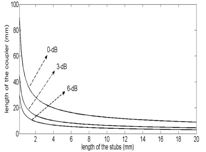
Fig. 3. Data for designing dimension of the proposed coupler on FR-4 substrate ( $\epsilon_r = 4.8$ ,  $h = 1.6 \text{ mm}$ ).
