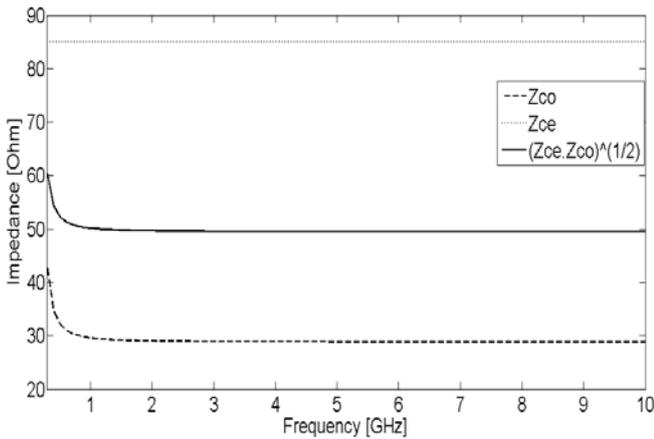
Fig. 5. Characteristic impedances of the even and odd modes.
