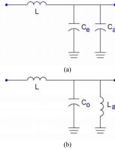
Fig. 2. (a) Even mode equivalent circuit of each coupled-line for one period, (b) Odd mode equivalent circuit of each coupled-line for one period.
