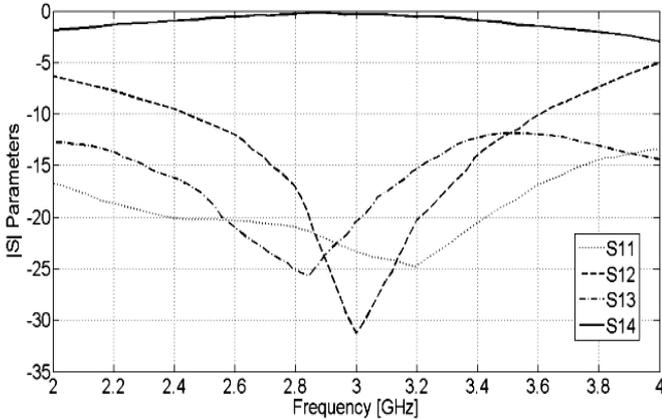
Fig. 6. Simulation results ( $|S|$ -Parameters) of the proposed coupler on FR-4 substrate ( $\epsilon_r = 4.8$ ,  $h = 1.6$  mm)
